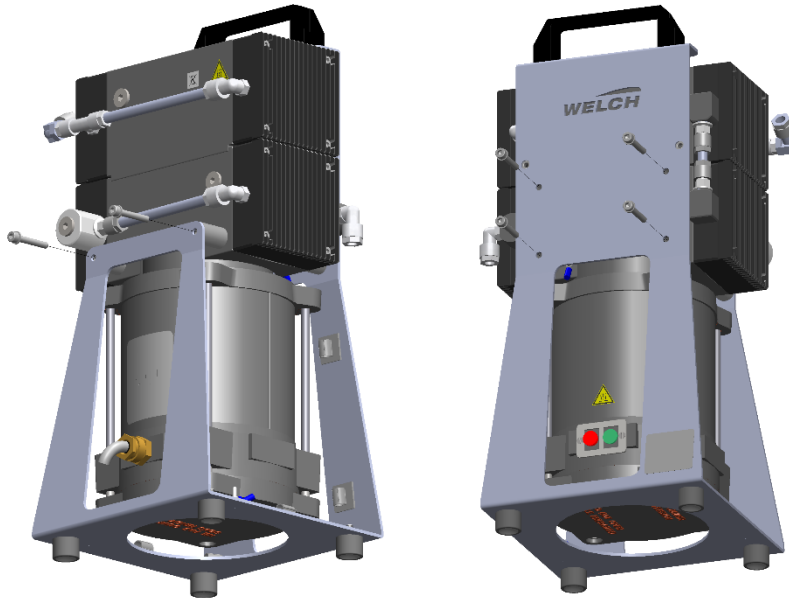
Fig. 8-1. Releasing the screw connection: back (left), front (right)
